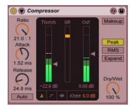
Above is an image of a compressor set to a very high 21:1 ratio and the "thresh" or threshold is set to -22.6 dB.
